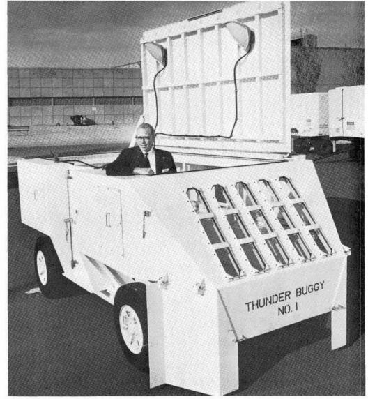
THUNDERBUGGY—Resembling an armored car or a tank, this vehicle designed by Dean Gladow of Test Range Department will be used as an instrumentation shelter during explosive tests in Area Y and Coyote Test Field.
